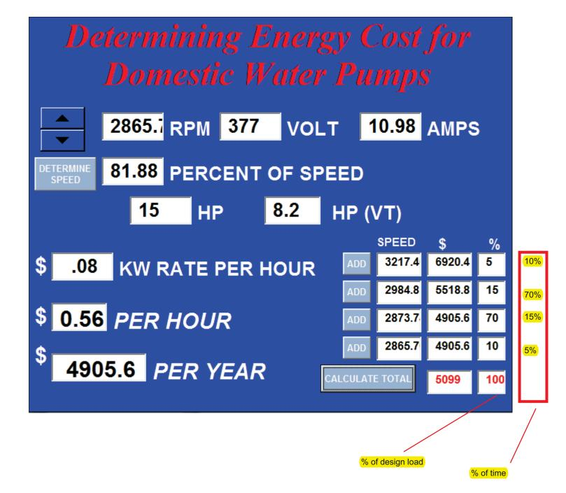
ENERGY CONSUMPTION/ COST TO OPERATE END SUCTION PUMP AT PROFILED LOAD
