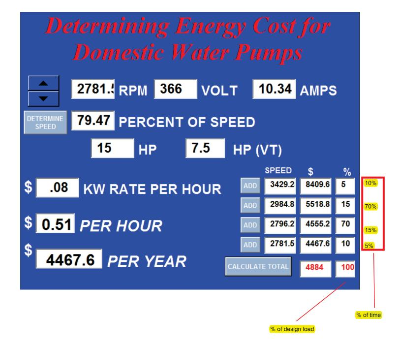
ENERGY CONSUMPTION / COST TO OPERATE MULTI-STAGE PUMP AT PROFILED LOAD
